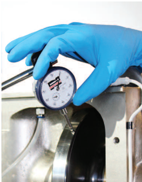
Adjust the dial or digital indicator until it makes uniform contact with the pressure roll and lock it in place by tightening the clamp.
