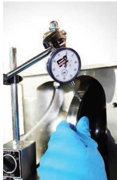
Turn the pressure roll slowly by hand to determine the run-out value.
