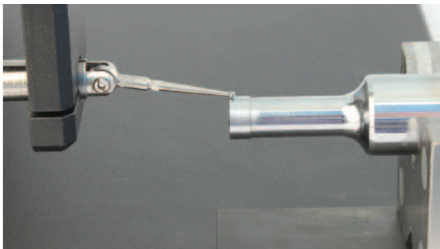
A tooling condition monitor [1] measures wear rings on the inside of a die, detects punch-tip wear, and predicts clearance issues by compiling micro-measurements and analyzing the data. The data enable you to forecast tool life by tracking wear between tools. The monitor is one of the few devices that measures die-bore wear and detects wear rings.
